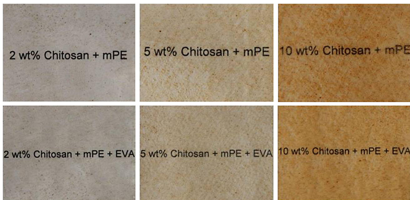
Fig. 3. Plasticized chitosan-based films for different chitosan content.
